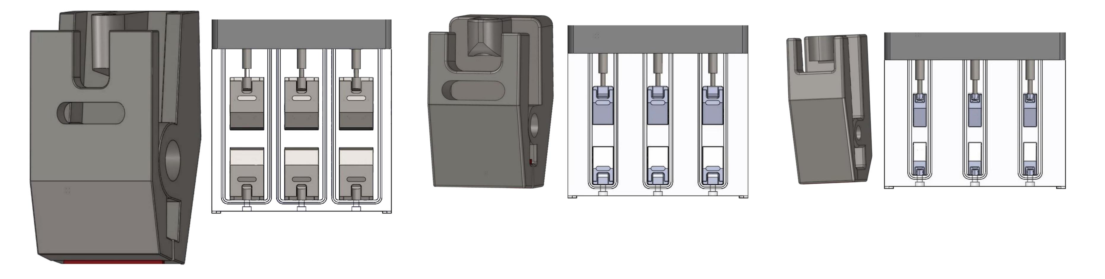
The MCJ1 Specimen Grips come in 3 standard sizes that are paired with matching specimen chambers. The clamping force of each grip can be adjusted by changing out the grip spring. Spring-closure grips ensure consistent clamping force from test-to-test and during each test. Customizations to the standard grips and chambers is readily available to meet research needs.
